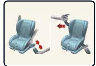
Securing a child restraint system with a lap/shoulder belt [4]
