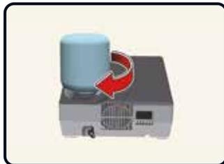
With the Tyre Mobility Kit you stay mobile even after experiencing a tyre puncture. After ensuring that the tyre is properly sealed, you can drive cautiously on the tyre (for a distance of up to 200 km (120 miles)) at maximum speed of 80 km/h (50 mph) in order to reach a service station or a tyre dealer to have the tyre replaced.
